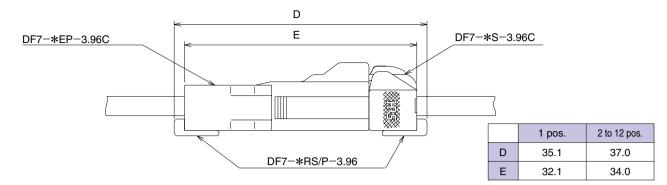
• Socket to In-line Plug Connection
